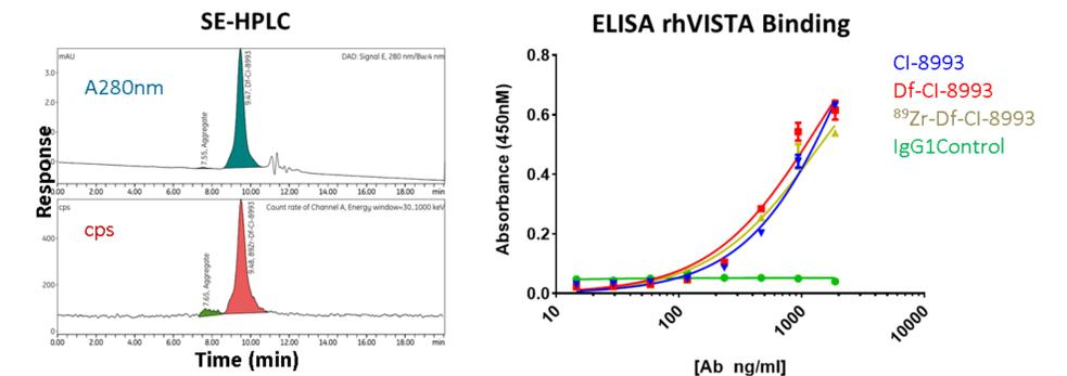
Figure 3. Left: Size exclusion (SE) HPLC A280 and counts per second (CPS) scintillation trace of <sup>89</sup>Zr-Df-CI-8993. Right: ELISA analysis binding recombinant human VISTA (R&D Systems).
