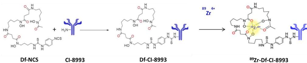
Figure 1. Schematic of radiolabeling reactions.
